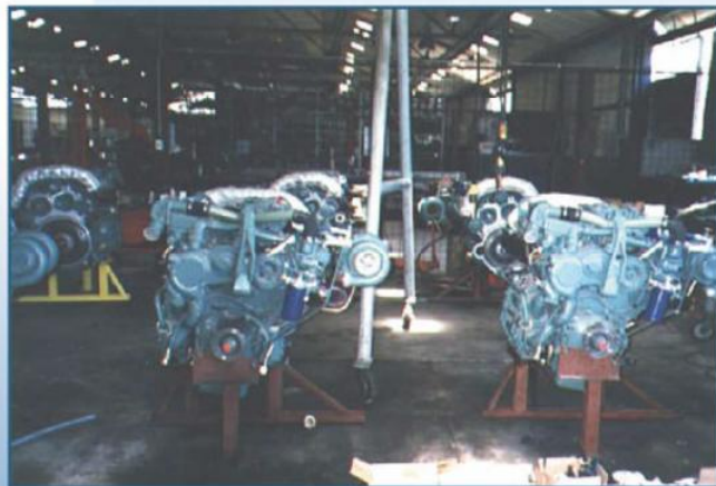
M-41 Engine assembly line
